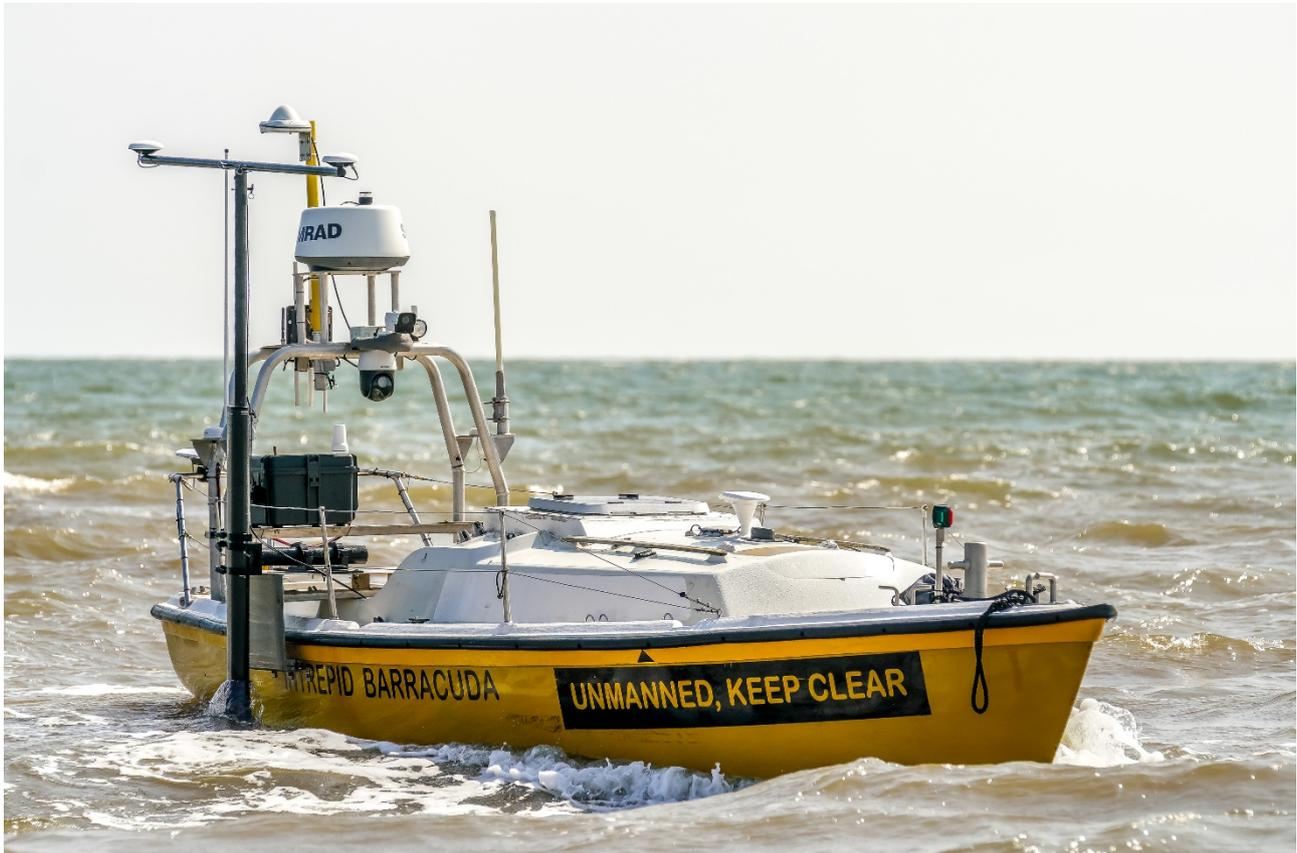
Intrepid Barracuda was converted from a 7m sailing yacht to an ASV (autonomous surface vessel). The yacht hull form with its proven sea-keeping has ideal smooth motion characteristics which provide a stable platform for mounting the bathymetric, communications and positioning systems necessary for conducting hydrographic survey.
